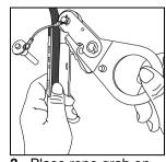
**3.** Place rope grab on rope with plastic roller pointing up.
